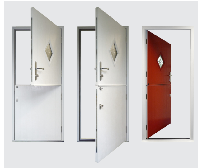
With the rack bolt (by others) engaged and all hooks retracted the door operates as a conventional door, releasing the rack bolt separates the upper and lower leaves, you can now choose to open the top portion only.
